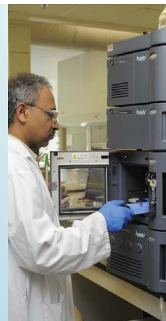
Insertion of samples in the sample manager of OICR's Ultra Performance Liquid Chromatography (UPLC) system
