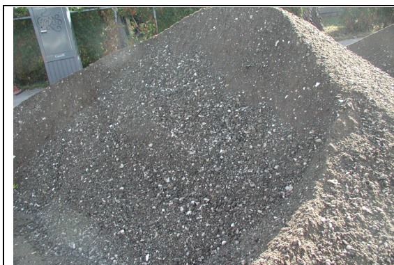
Photograph 3-16: Waste Ceramic Material Stockpiled waste ceramic material (15%) and crushed concrete Granular A (85%) RCM.
