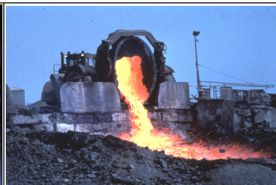
Photograph 3-11: Steel Slag Dumping molten steel slag from a transporter at a cooling pit (1990s).
