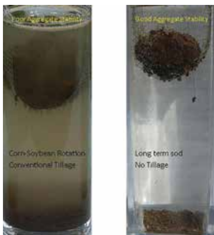
Photo 8–12. Aggregate stability demonstrated with a good and poor crop rotation.
