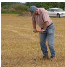
Photo 8–3a. Identify parts of the field with potential compaction problems by using a tile probe or flexible rod.
