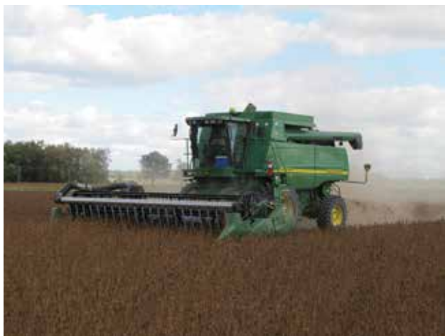
Photo 2–8. Combine with air reel to minimize losses.
