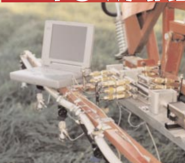
Rear view of sprayer showing metering pump apparatus with supervisory control computer and injection nozzles on spray boom.
