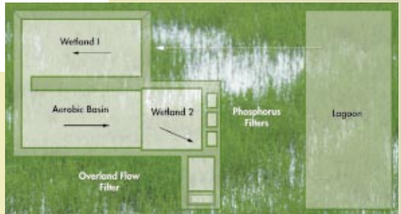
Fig. 1. The experimental constructed wetland at Alfred consists of two free-surface wetland cells, an aerobic pond, an overland flow and phosphorus adsorption filters. It will begin treating 5% to 15% of the wastewater flow entering the Alfred municipal lagoons in summer 1999.
