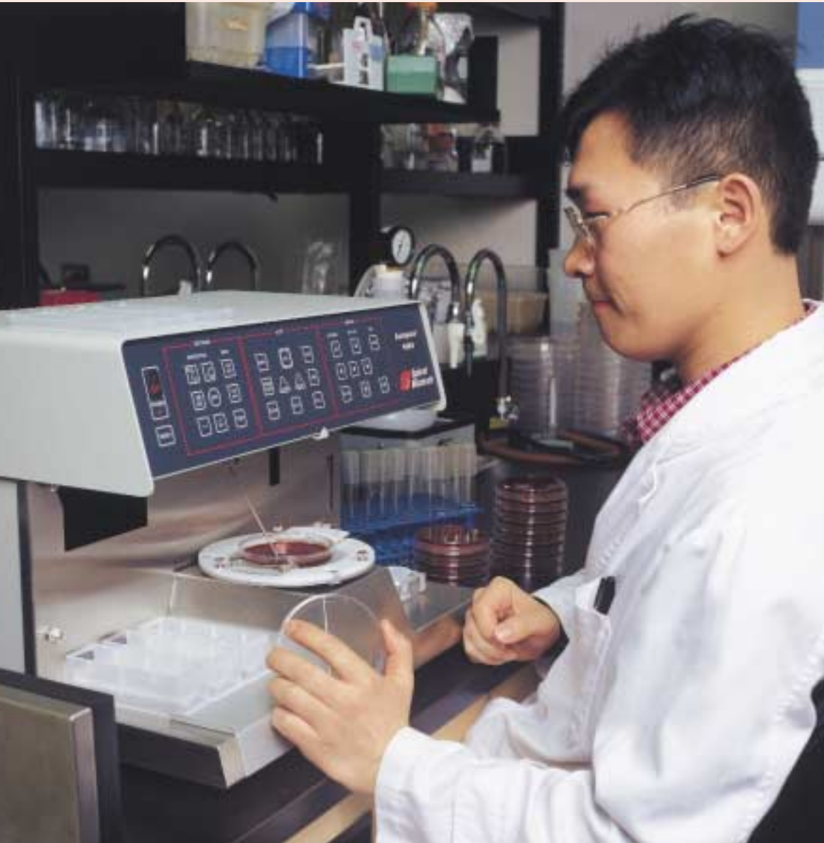
Min Seok Chae, a graduate student in the Department of Food Science, University of Guelph, uses an automated system (Spiral Plates) to count bacteria grown in a biofilm.
