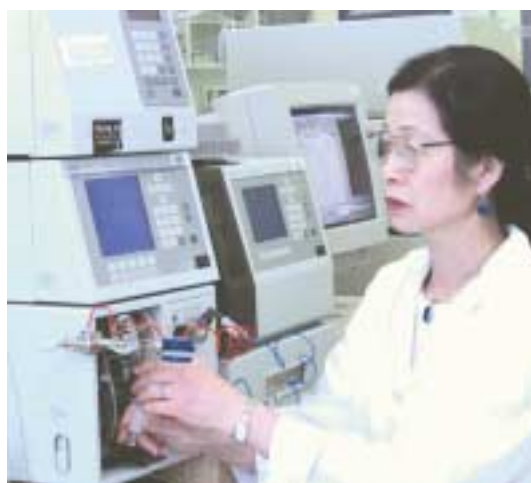
Fig. 1. Dr. Chung-Ja Jackson uses high performance liquid chromatography to measure isoflavone levels in different soybean varieties.
