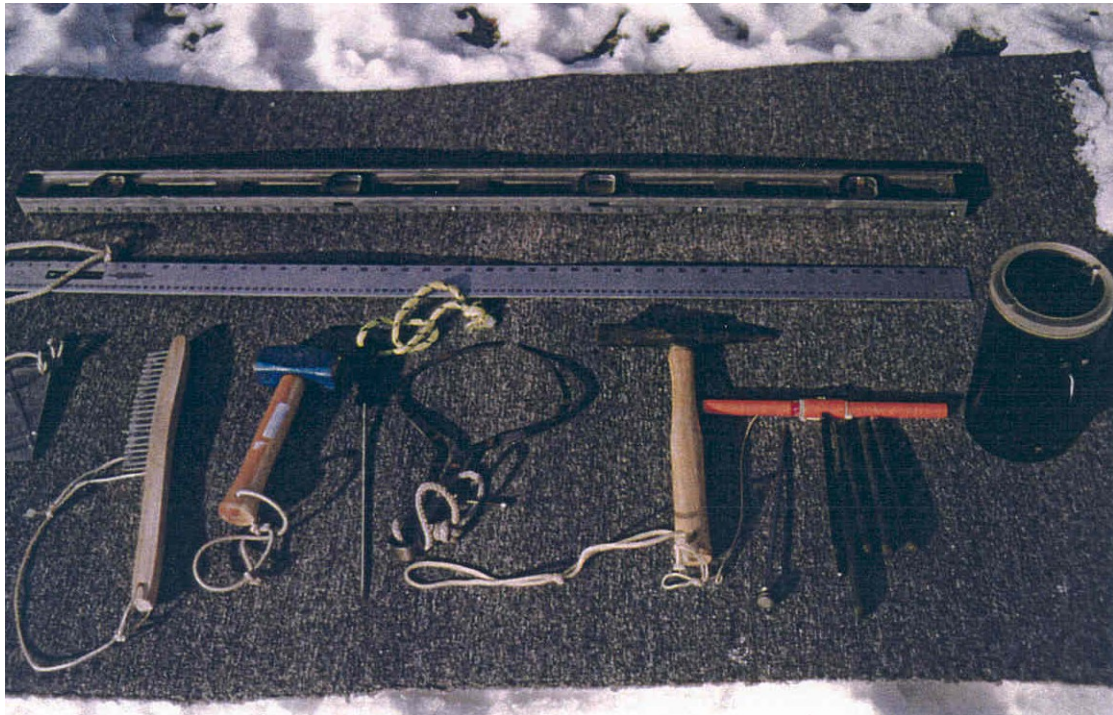
Figure 2.1 Typical Hand Tools for Underwater Inspection
