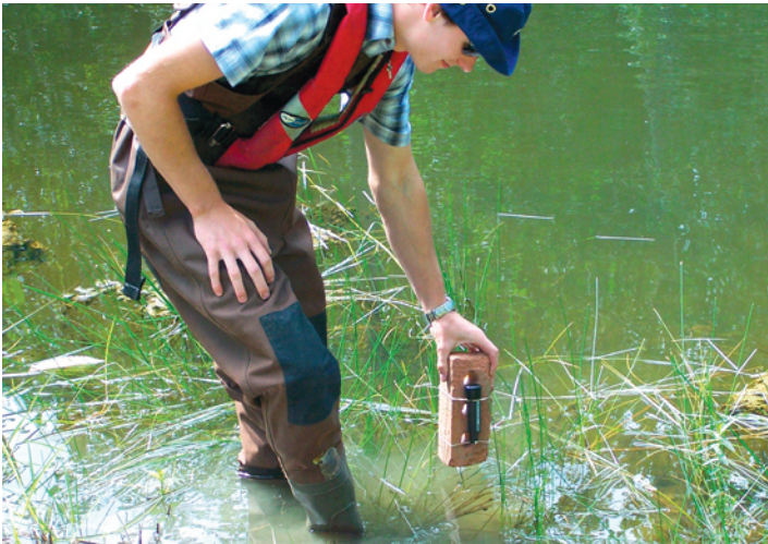
Technician Andrew Hibma deploys a temperature data logger
