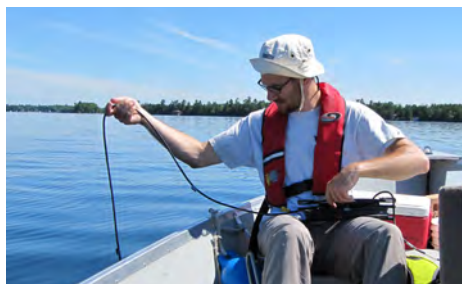
Resource Technician Ben O'Reilly uses a YSI handheld multiparameter meter to measure dissolved oxygen, pH, conductivity, and temperature in Balsam Lake. Water samples are also collected and measured for total phosphorus (TP), total suspended solids (TSS), metals, anions, and all chemical forms of nitrogen, including total Kjeldahl nitrogen (TKN), total ammonia ( \text{NH}_3 + \text{NH}_4^+ ), nitrite ( \text{NO}_2^- ) and nitrate ( \text{NO}_3^- ).
