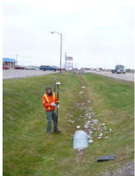
Paul Buckley, Kawartha Conservation GIS/Survey Technician, surveys culverts and bridges in the Ops Drain/Jennings Creek watershed for a floodplain mapping and engineering project.
