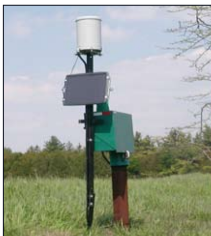
PGMN rain gauge installed in 2007.
