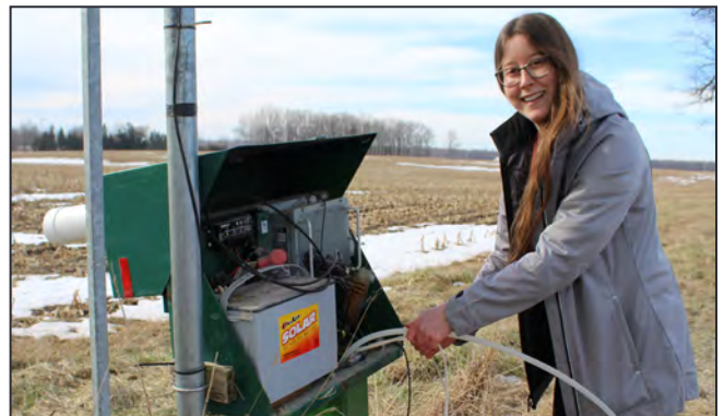
Assistant Water Resources Technician Christie Brown measures groundwater levels at one of the monitoring wells in the watershed.
