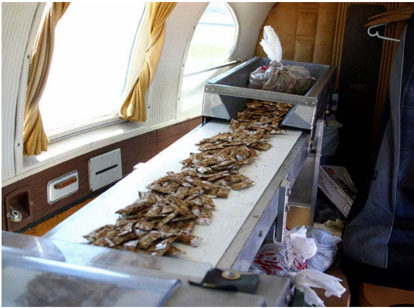
Figure 4. Coated sachet baits being distributed from the Navajo.
