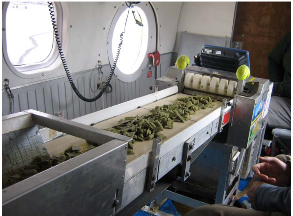
Figure 5. Rabies bait dropping machine loaded with ultra-lite baits in the back of a Twin Otter.
