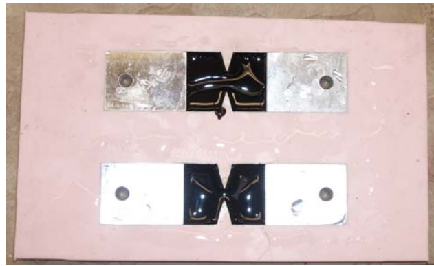
Figure 9 – Silicone Mold with Asphalt Samples in Aluminum End Pieces
