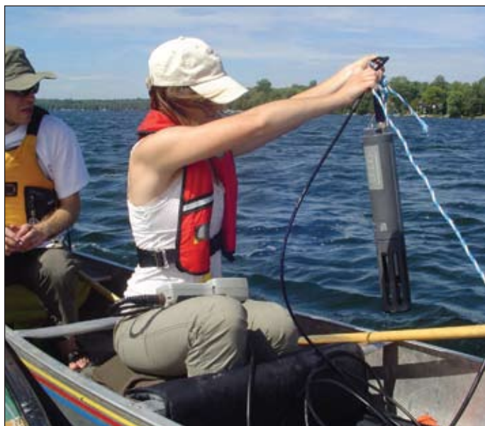
NVCA staff Ian Ockenden (left) and Natosha Fortini conduct dissolved oxygen profiling in Bass Lake.
