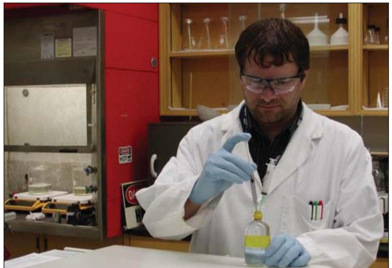
A water sample is tested for nitrate levels in a Ministry of Environment lab.
