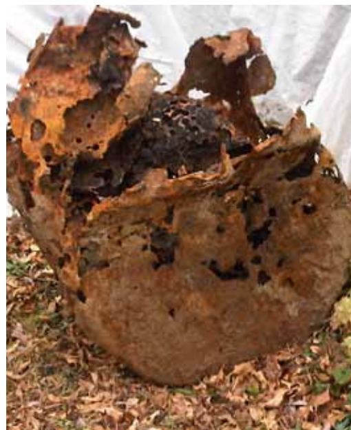
A septic tank removed by the stewardship program.
