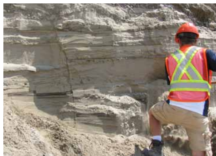
A geological assistant inspects layered sands and gravels within the South Simcoe County study area that may yield groundwater sources for municipal water supply.
