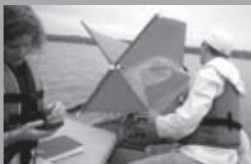
A data gathering device called a drogue is prepared for launch into Lake Ontario. The drogue gathers information on currents and winds which is then used to determine water flows into the municipal intakes along Lake Ontario and the St. Lawrence River.
