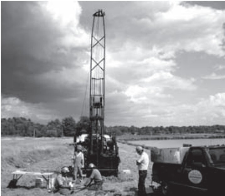
Drilling boreholes was one of the ways to determine what is happening with the groundwater in the Lansdowne area. Lansdowne is one of the few communities in the Cataraqui Source Protection Area that relies on groundwater for its municipal water supply.
