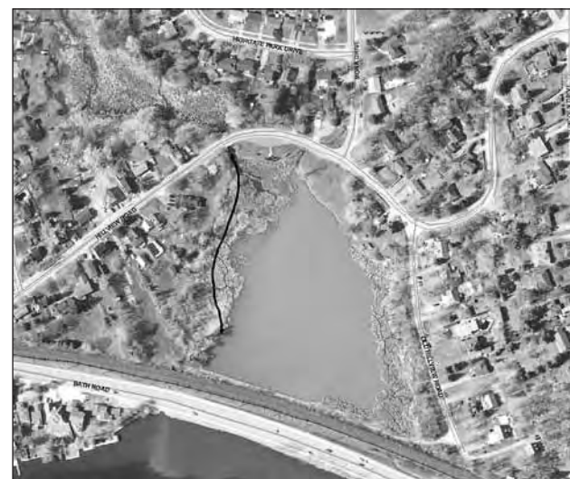
The dark line on this aerial photo shows the location of the dredging that will take place on Highgate Creek this winter. The dredging will ensure that the water flowing through the creek flows into Collins Bay more quickly.
