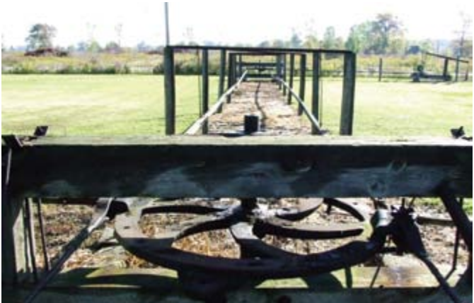
Field wheels (shown here) and jerker lines operate on the Fairbank Oil Properties today, much as they did in the 1860s. Photo: Oil Museum of Canada.
