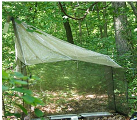
Malaise trap erected in forest habitat.
