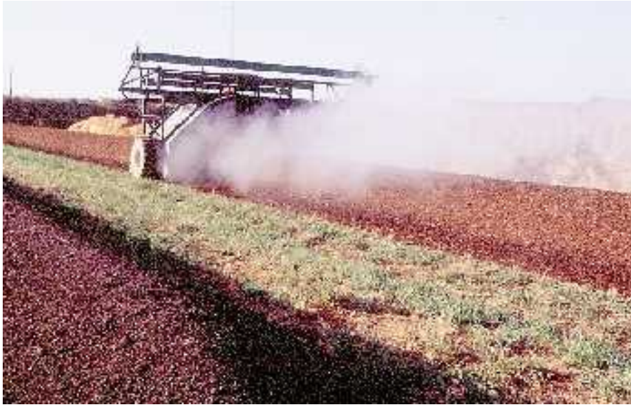
Compost turner mixing pile to distribute moisture and heat evenly. Note the steam released from the centre of the pile
