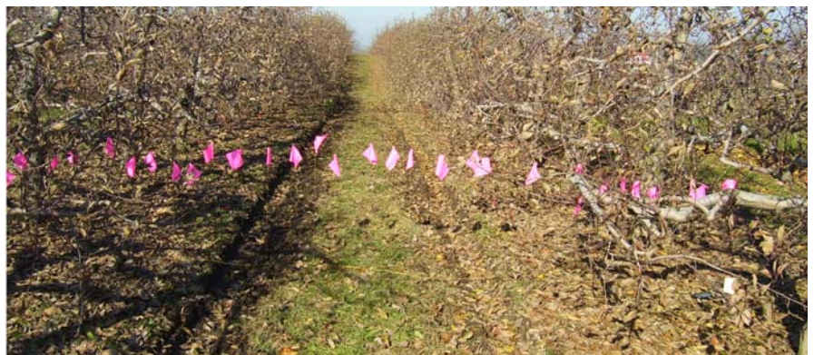
Figure 2 – Flag height reveals the depth to which a wire rod can be pushed into the soil in the space between tree rows. The higher the flag, the more compact the soil is.
