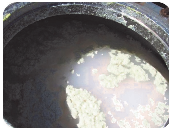
Figure 3. Physical incompatibility in the tank
