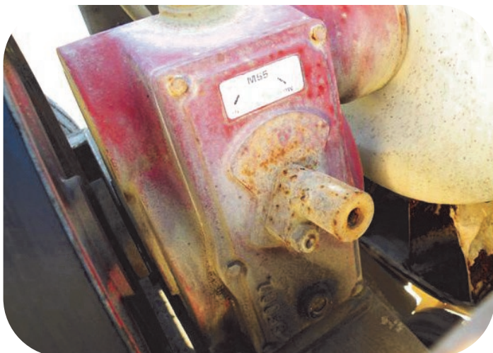
Figure 1. It takes time and elbow-grease to get seized parts, such as this fan gear box, moving again. Plan for half-a-day per sprayer when performing your seasonal start-up, and be sure you have a source for replacement parts.
