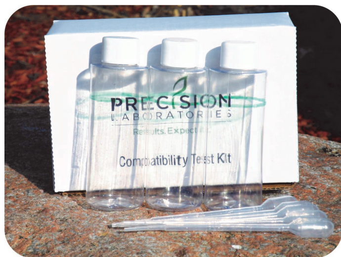
Figure 5. Contents of a commercially-available compatibility test kit
