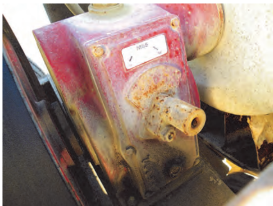
Figure 1 – It takes time and elbow-grease to get seized parts, such as this fan gear box, moving again. Plan for half-a-day per sprayer when performing your seasonal start-up, and be sure you have a source for replacement parts.
