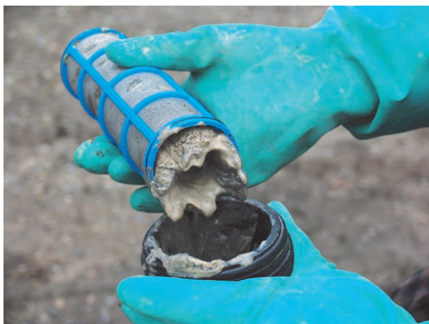
Figure 8: Inline filters shouldn't look like this. This was a serious tank-mix incompatibility issue.
