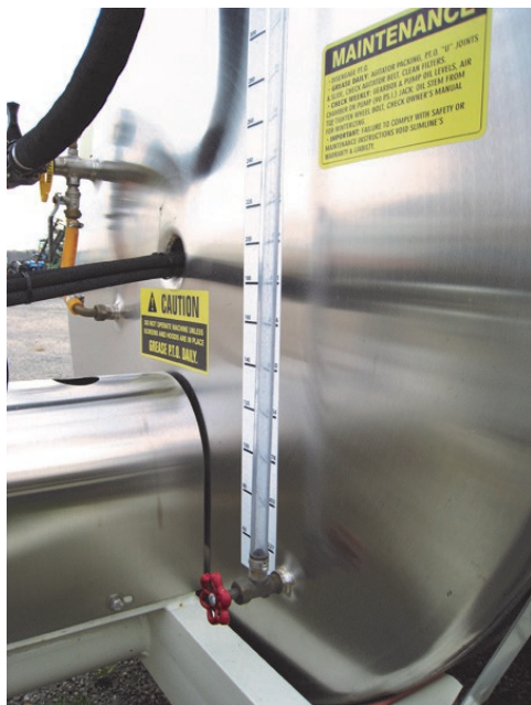
Figure 9: This plastic 'sight glass' indicates how full the tank is. They become opaque and unreadable in a season or two, but they're very easy to replace.
