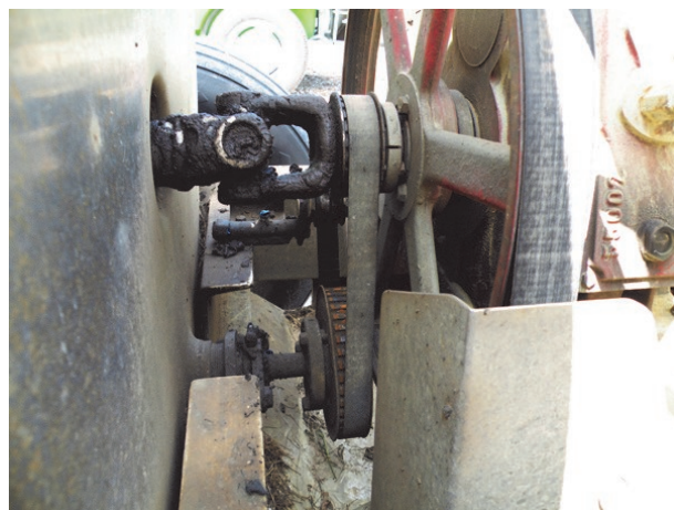
Figure 10: Check the belt alignment. If the belt is not exactly true (i.e. in line), it will not operate efficiently and may wear out more quickly.
