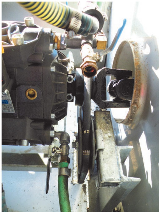
Figure 11: Universal joints seize and break more often than you think. Check and grease them regularly.
