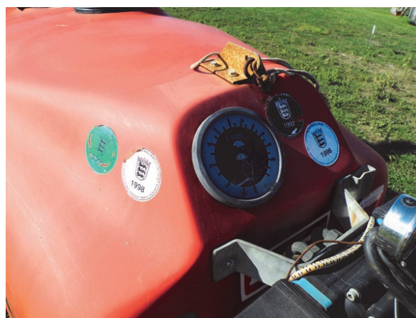
Figure 1: This used Myers sprayer was imported from Europe by a vineyard in Prince Edward County, Ontario. Many European countries require regular sprayer maintenance inspections before the operator can use them. The stickers on this sprayer show that it was maintained and calibrated correctly. In certain countries, sprayers that are not compliant are “grounded” until the issue is remedied, and the owner is charged a hefty fine. We don’t require this level of compliance in North America... yet.
