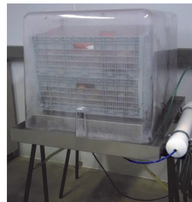
Figure 1: SafePod technology with apples. SafePod measures the fruits' response to atmospheric stress by monitoring its respiration rate, which will be the primary metabolic process to change when oxygen becomes too low and there is potential for fruit injury. This allows for the lowest safe oxygen concentration to be used in apple storages.
