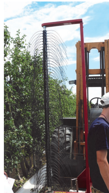
Figure 1. A Darwin string thinner used to mechanically thin blossoms
