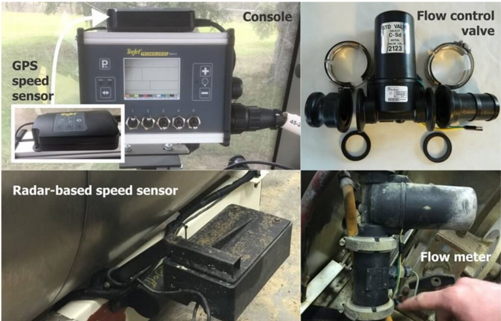
Examples of rate controller components.
