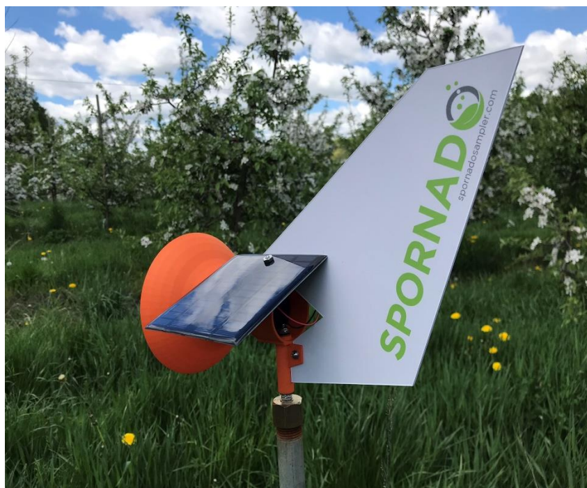
Figure 2. Enhancements to the Spornado air sampler includes the addition of a solar-powered fan to increase air passage through the collection cassette which improves spore detection in an orchard setting.
