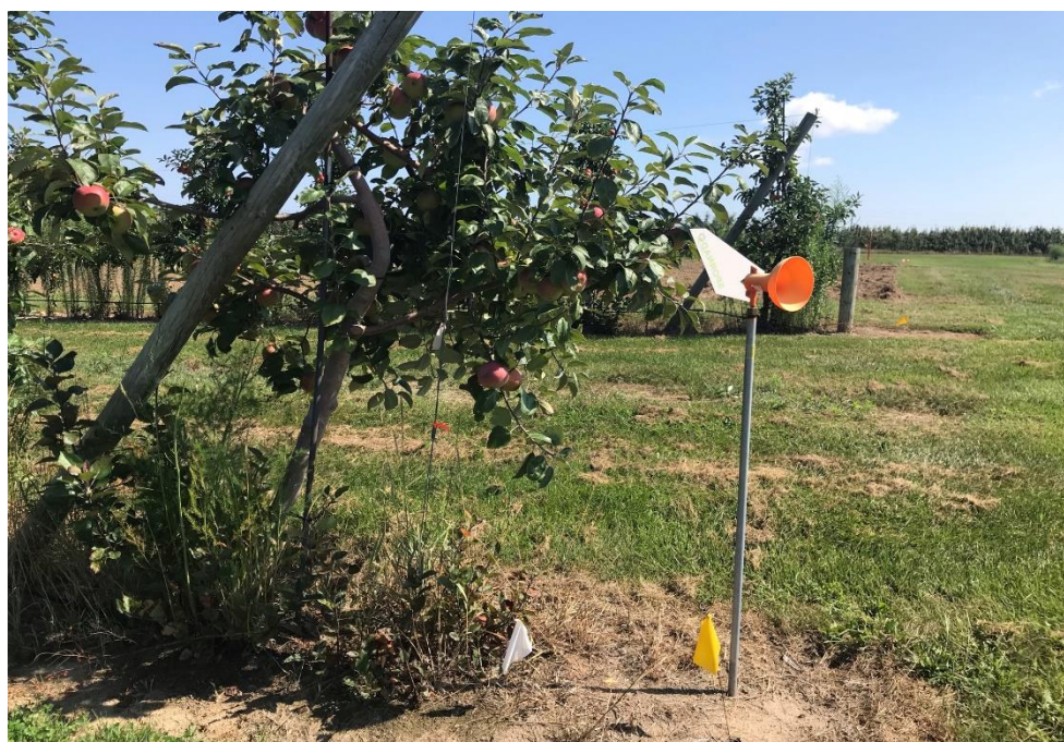
Figure 1. Passive wind-powered Spornado air sampler placed at the end of a row of Ambrosia within an orchard with a history of apple scab. Spores carried by wind are collected from the air through the orange funnel onto sample cassettes which are then shipped to a laboratory for analysis.
