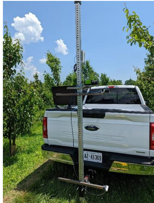
Figure 2. Data collection system mounted on a truck
