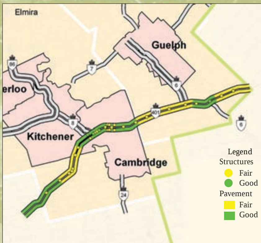
An example subcorridor indicating asset condition.
