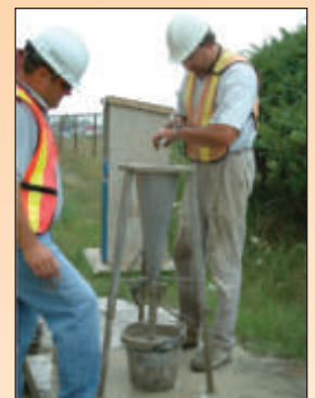
Right: Using a V-funnel to evaluate the flowability and stability of SCC in a field test.
