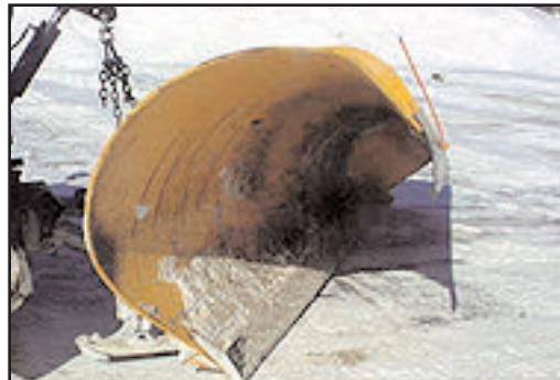
Figure 1. Standard steel blade composed of a straight steel piece attached to the bottom of plow
