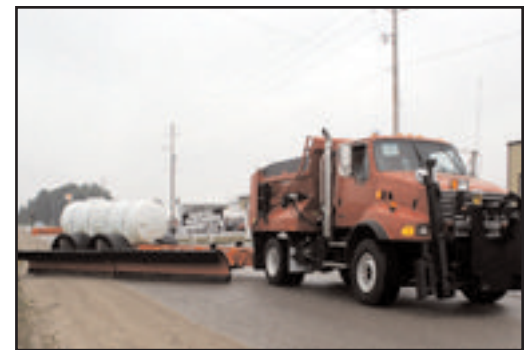
Figure 4. Viking trailer with multiple plows
