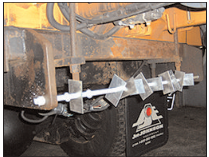
Figure 1. Coupons mounted under the body of winter maintenance vehicles
