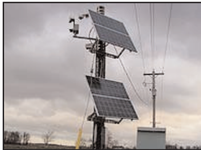
Figure 1. Solar panels are the power source for MTO's Total Monitoring System
