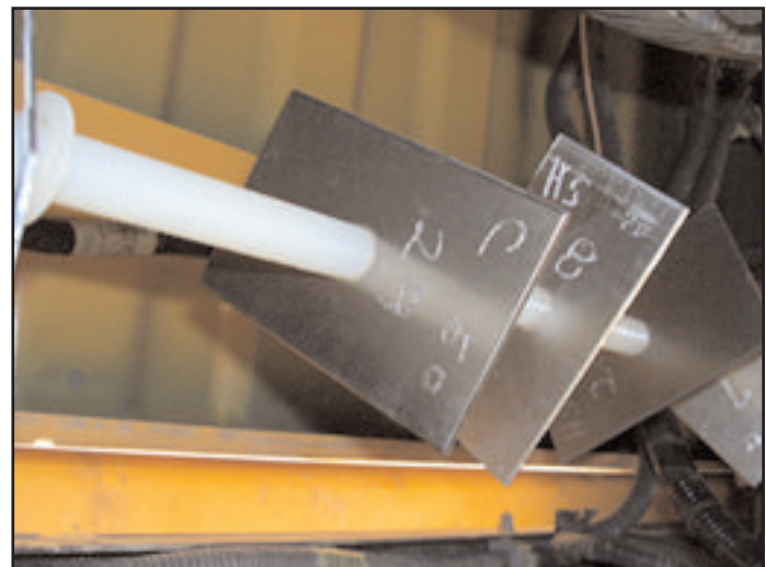
Figure 2. Detail of metal coupons exposed to areas with WRMLs containing different levels of corrosion inhibitors
