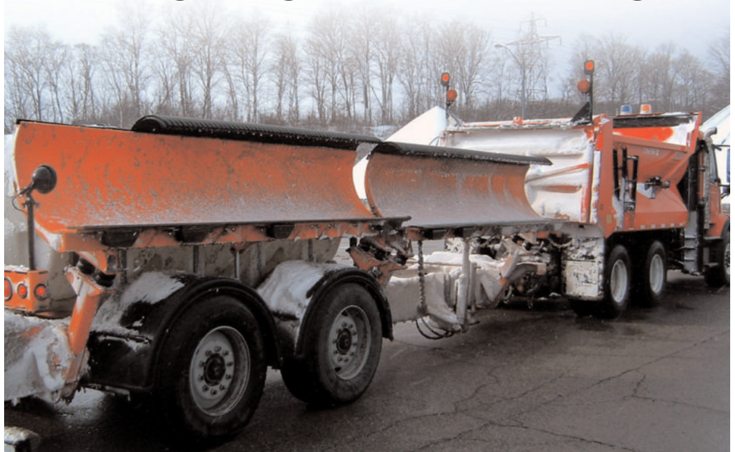
Standard blades in the Viking trailer multi plow work independantly of each other to plow lanes
