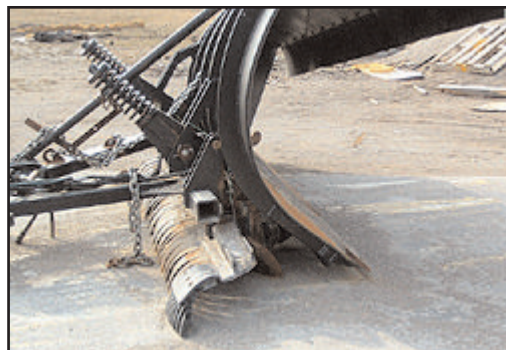
Figure 3. Viking Double Plow blade (side) is formed by a standard blade and trailing sweepers
