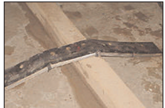
Figure 2. The Joma blade's flexibility, attributed to rubber mounted steel segments, is demonstrated over a plank
