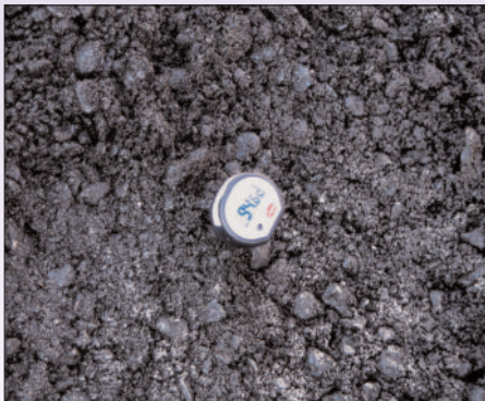
Temperature of Warm Asphalt was ~95° C after production trial.
