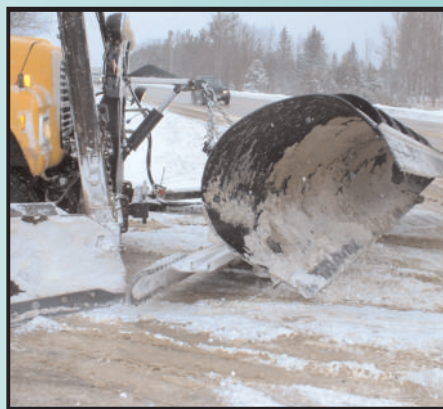
The Two Stage blade features a smaller trailing blade with flexible segments that clean off loose snow and clear slush.
