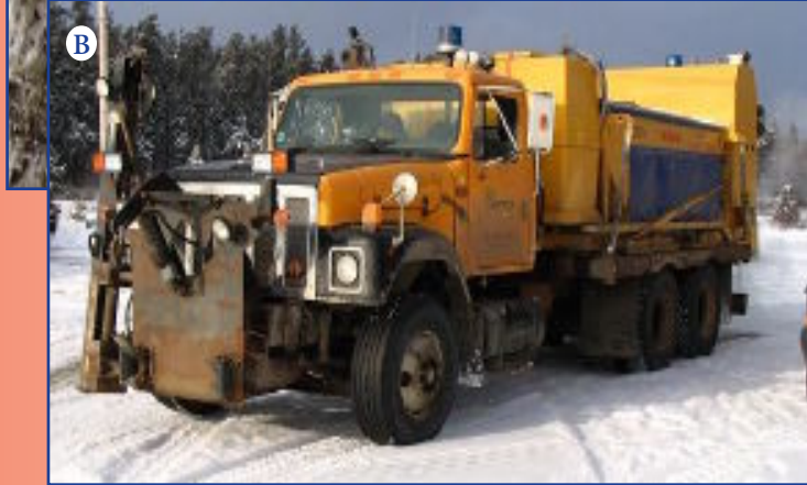
B: The hot water sander design uses a modified version of a traditional salt spreading truck.
