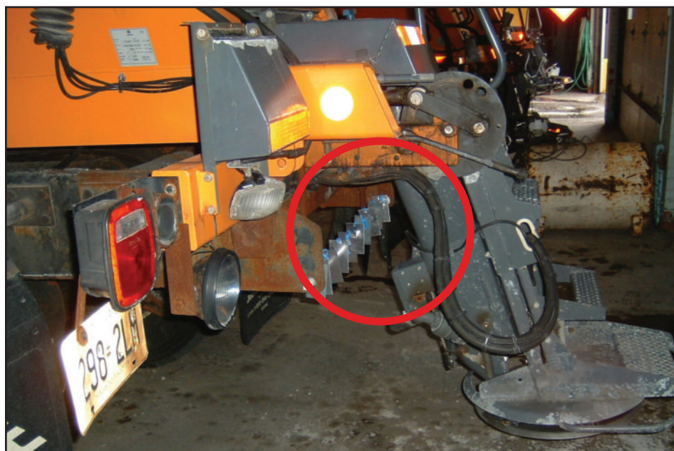
Figure 3: Coupons to be tested were also set up on road maintenance vehicles.
