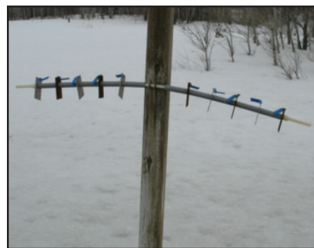
Figure 1: Alternating steel and aluminium coupons suspended on threaded nylon rods for field testing in Ottawa.
