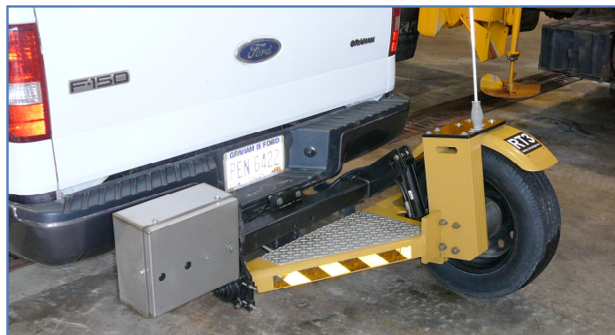
The Halliday RT3 Friction Meter is used to model relationships between surface conditions and surface friction during winter storm events.
