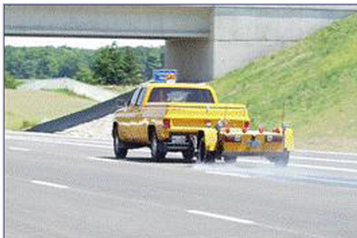
Demonstrating controlled friction on a simulated wet highway surface
