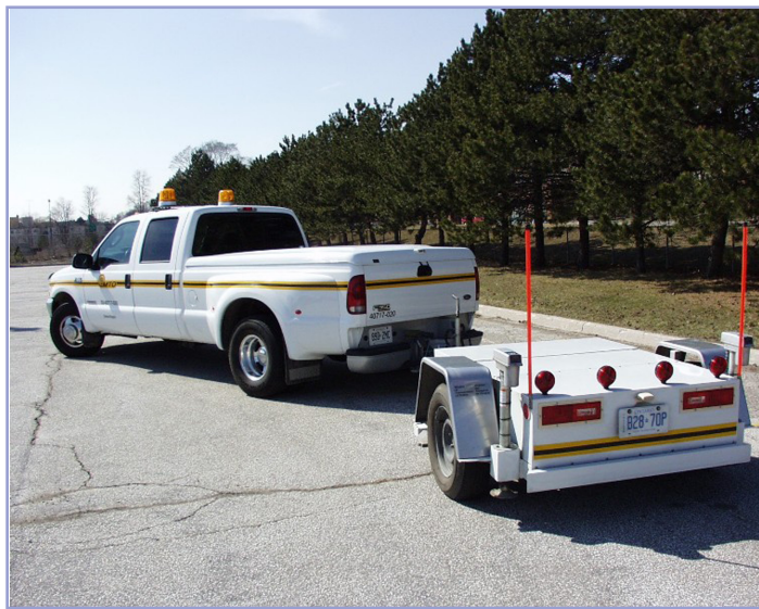
An ASTM E-274 Brake Force trailer unit connected to a standard MTO fleet truck.
