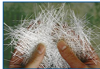
Chopped fibreglass strands, 5 to 10 cm in length, used for SAMI application.
