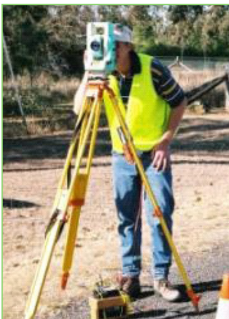
Figure 4: A Total Station is the traditional survey instrument used for conducting topographic surveys.
