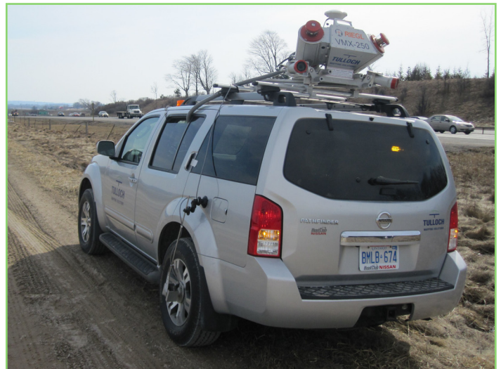
Figure 1b: Mobile LiDAR System Mounted on an SUV
