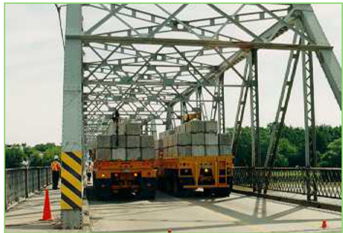
Figure 2: Test trucks on bridge
