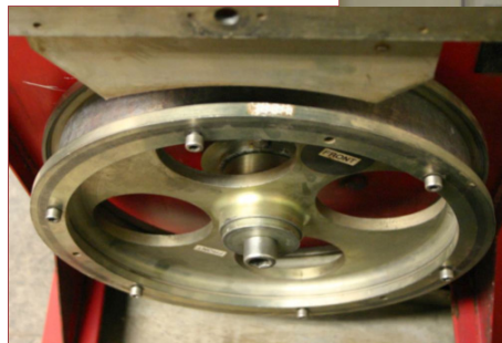
^ Figure 2: PSV machine, side view showing wheel onto which the sample coupons are mounted
