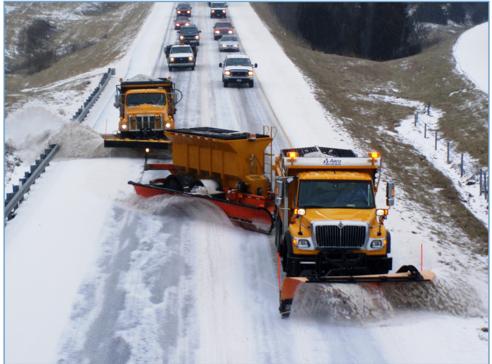
A tow plow, and regular snow plow, in "echelon" operation.
