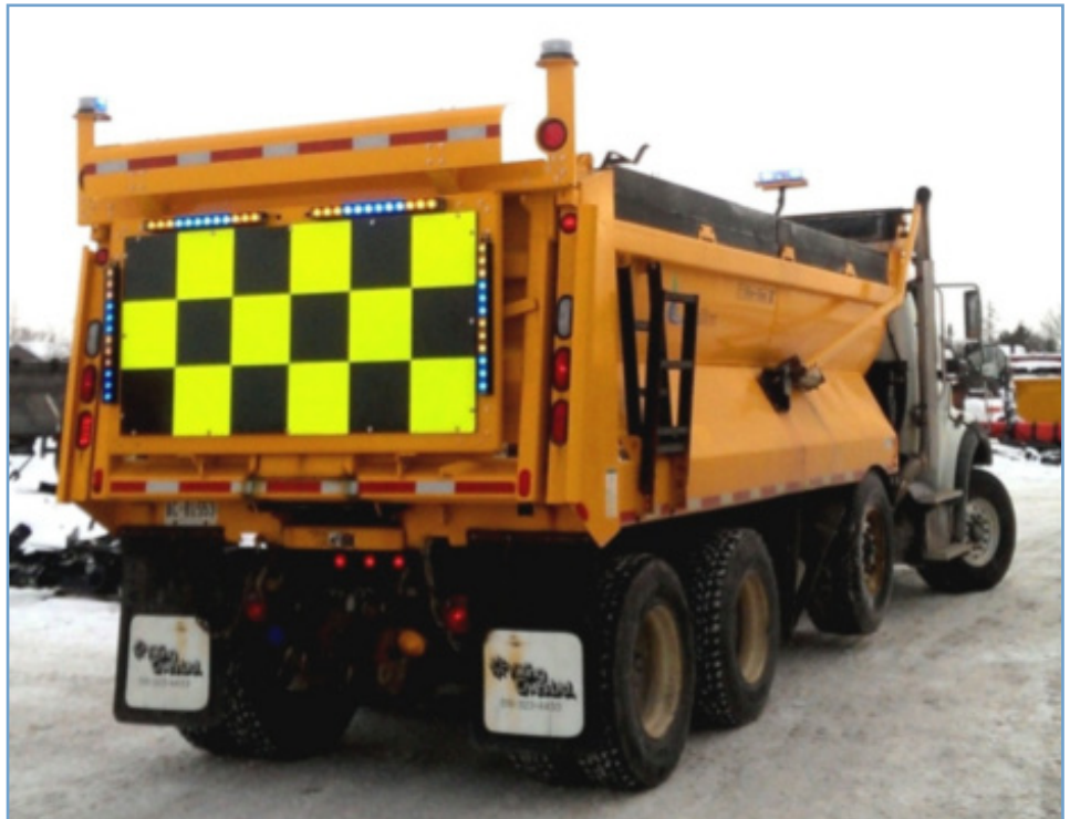
The new MTO standard for winter maintenance equipment lighting and visibility
