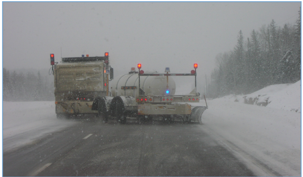
A tow plow in operation, with the plow extended out, to the right. The increased clearing path is evident.
