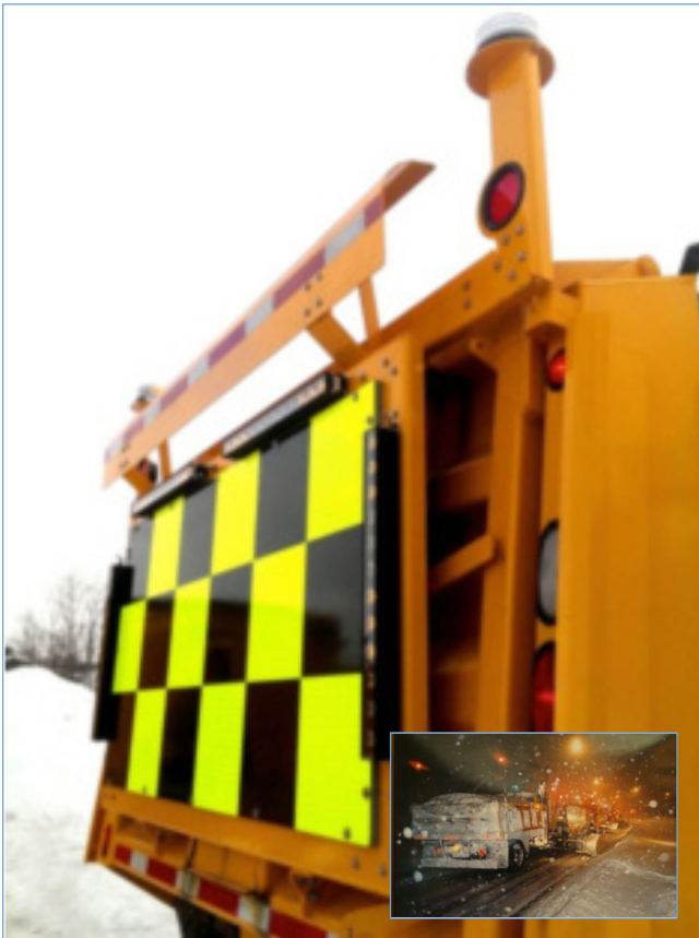
Air foils reduce snow, slush, and salt build-up on the rear lights and panel.
