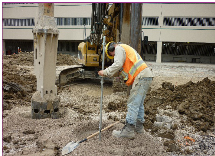
Figure 5: Conducting the Dynamic Cone Penetrometer Test (DCPT) with hand-held equipment.
