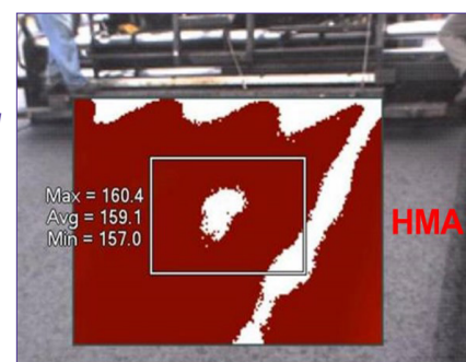
Figure 1a: Hot Mix Asphalt thermal image showing temperature ranges from a minimum temperature of 157.0°C to maximum 160.4°C, averaging 159.1°C.
