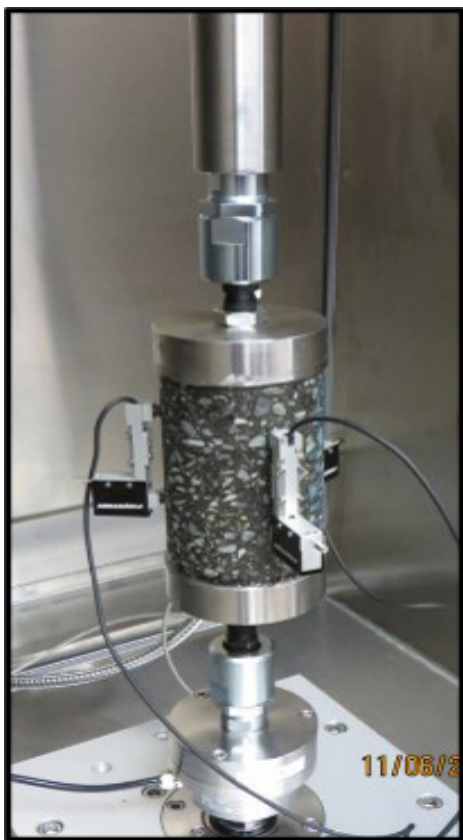
Dynamic Modulus. Part of the bituminous mix evaluation equipment.
