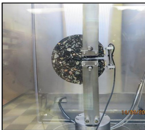
Disk-Shaped Compact Tension (DCT) - part of the bituminous mix evaluation equipment.
