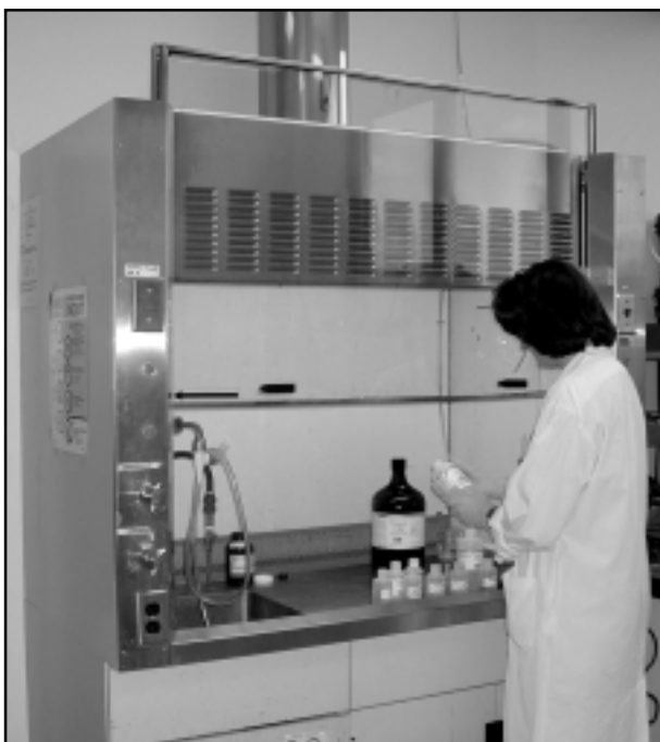
FUME HOOD: A University of Ottawa researcher dispenses flammable liquids safely in a fume hood.
