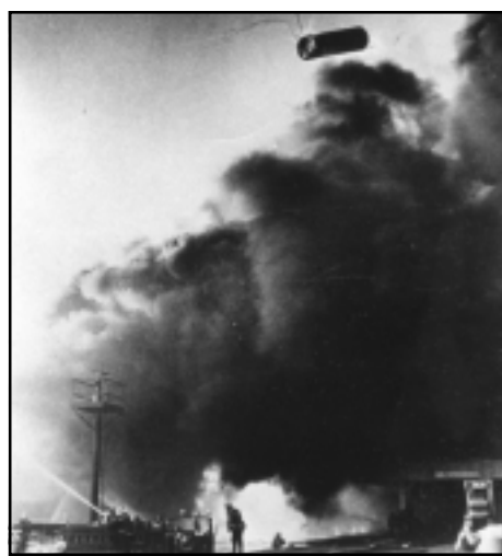
ROCKET: Inadequate emergency relief venting can cause tanks to explode violently or rocket great distances.*
