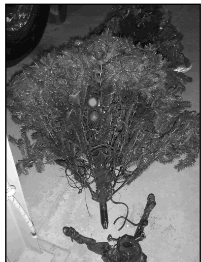
If you look closely, you can see the stand, which the tree was in, is melted, and the base of the tree is singed.
