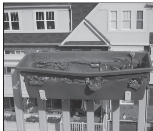
A picture of a pot that contained potting soil. A fire occurred when the occupant attempted to extinguish a cigarette butt in the soil. Photo submitted.
