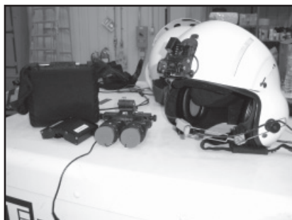
Apparatus for the night vision includes the aviation helmet and night vision goggles. Photo submitted by Travis Moffatt, MNR.
